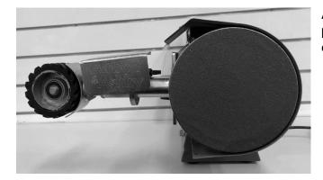
Attach the abrasive disc to the backing plate. Hold firmly for a few seconds to ensure the adhesive activates.
