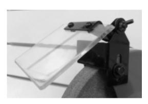
Use the wing nut (D) and 1 x washer (B) secure the eyeshield to the bench grinder allowing no more than 2mm gap between the grinding wheel and bracket (A)
