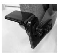
Attach the tool rest (A) to the bracket (B) using the long fastener (G) and the Large Washer (C) and wing nut (D). then attach this to the bench grinder using the 2 x small washers (E) and 2 x short fasteners (F), allowing no more than 2mm gap between the grinding wheel and tool rest (A).
