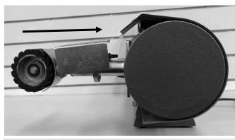
Push against the contact wheel towards the drive pulley to retract the extension arm and place the linishing belt over the main wheel and the contact wheel. Refer to the inside of the belt for the correct installation direction of the belt.
