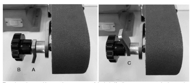
Turn the unit on and inspect the movement of the belt. If adjustments are required move the lever into the loose position (A) To correct any tracking concerns simply turn the knob (B) to adjust the tracking and once adjusted lock the lever gently back into place (C).
